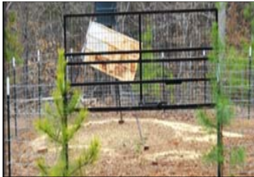
Figure 27: Remote controlled door design triggered by a cellular signal.
