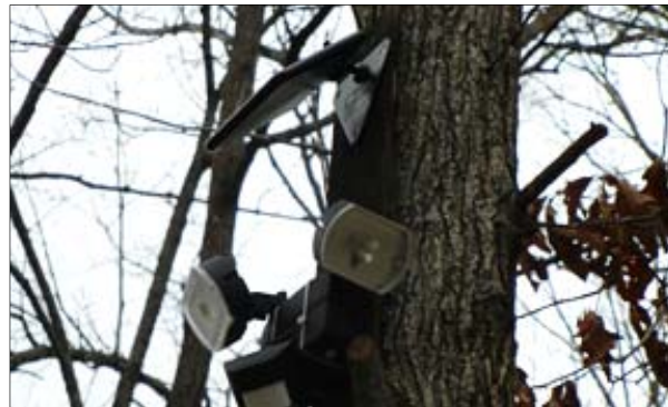
Figure13: Solar powered flood lights with a motion detector mounted to a tree (survival-gear-guide.com).
