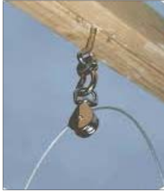
Figure 38: A pulley and S-hook used for guillotine gates.
